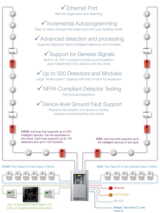
Diagram represents an iO500 system wired for Class A operation with a full complement of option cards.
